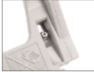
Screw boss completely restored. Use custom machine screw for reassembly.
